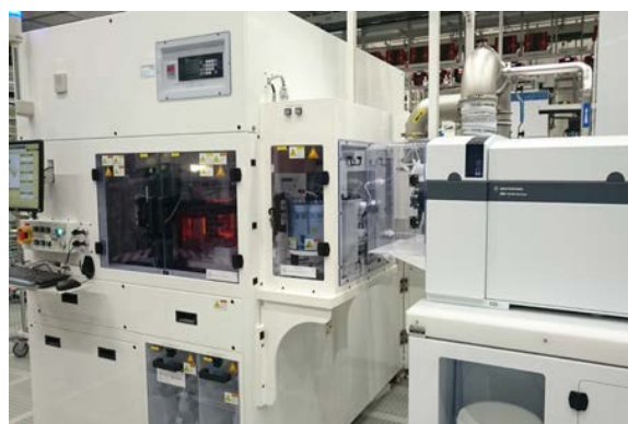
Expert PS fully automated VPD-ICP-MS system manufactured by IAS Inc. that was integrated with Agilent 8800 ICP-MS/MS. The figure was provided by ST Microelectronics (Crolles, France)
